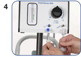
Attach the spray set to regulator. Connect the clear hooded luer connector on the tubing set to the male clear gas port on the regulator. Connect the blue male luer connector on the tubing set to the female luer blue vent port on the regulator.
