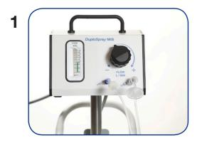
Check the gas flow meter on regulator before inserting applicator into trocar. Maximum flow rate = 2.0L/min; recommended spray distance 3cm (range 2-5cm).
