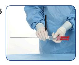
Push the snap lock all the way down to securely fasten the applicator to the syringe luers.
