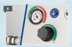
Check the gauge on the EASYSPRAY device for the appropriate pressure range of 1.5-2.0 bars (21.5-28.5 psi, green range). Adjust pressure setting by turning the black pressure control knob.
