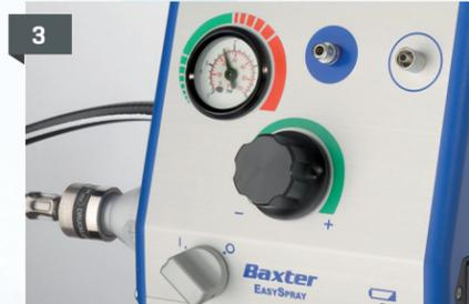
3 Attach connection tube from side of the EASYSpray Regulator to a propellant gas source (ranging from 3.5-7 bar / 50-100 psi). Use compressed medical air or nitrogen only, do not connect to an oxygen source.
