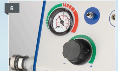
6 Check the gauge on the EASYSpray device for the appropriate pressure range of **1.5-2.0 bars** (21.5-28.5 psi, **green range**). Adjust pressure setting by turning the black pressure control knob.
