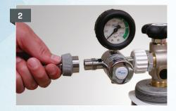
Adjust CO<sub>2</sub> source pressure to 100 psi / 7 bar (+/-5). The pressure gauge on faceplate of Regulator should indicate 18-22 psi/1.24 - 1.5 bar or in green zone.
