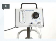
While depressing foot pedal, adjust gas flow rate to 1.0-2.0 liters per minute. Check gas flow by noting height of ball in flow gauge while stepping on foot pedal.
