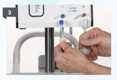
Attach spray set to regulator. Connect the blue vent line filter to the blue female luer and the clear gas line filter to the clear male luer on the regulator.
