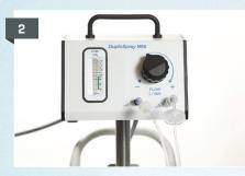
Check the gas flow gauge on the regulator before inserting applicator into trocar. If flow level ball does not move when foot pedal is pressed, the applicator is clogged and should be replaced.
